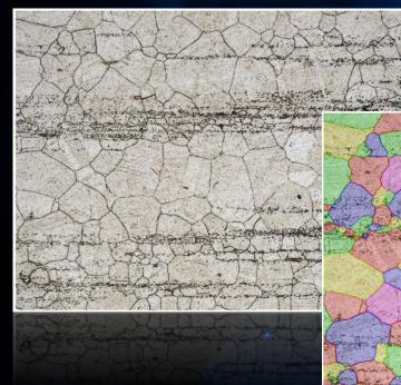
Al capabilities can automatically and correctly segment grains even on scratched or similarly damaged samples.
